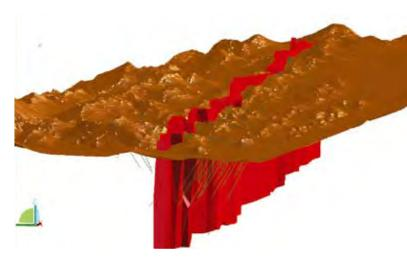
Figure 11. Isometric view of the design drill holes intersecting the Klondyke Shear.
