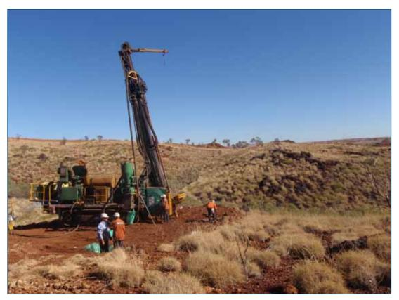
Photograph 5 RC Drilling Oakover Project
